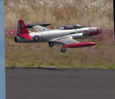
The Lockheed T-33 Shooting Star (or T-Bird) is an American subsonic jet trainer. The two-seat T-33 jet was designed for training pilots already qualified to fly propeller-driven aircraft.
